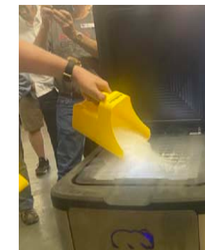
The process uses dry ice pellets for the blasting medium.
