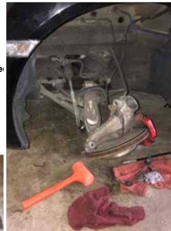
Driver side front strut removed
